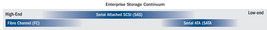
Figure 3: SAS will become the technology of choice for most storage needs, while coexisting with FC and SATA for very high end, or very cost-conscious requirements.
