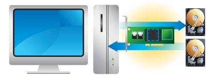
There are two types of controller cards: Host Bus Adapters (HBAs), and RAID controller cards.
