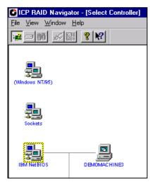
After the protocol was selected, select the system which contains the ICP Controller and afterwards the ICP Controller itself. The selection and de-
