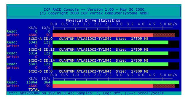
After selecting one of the Drives Statistics ICPCON displays a list of all Drives of this level (for this example the Physical Drives, i.e., level 1). In addition to the performance report on the Drives, you are given additional information on each device. The ICP I/O channel the hard disk is connected to, which ID the hard disk has, the name of the hard disk, the gross
