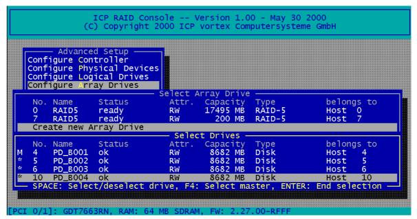
The "M" means Master. For a striping array (RAID 0, 4, 5, 10), this is the first Logical Drive in the array. For a RAID 1 (mirroring) array this is the Logical Drive which contains the valid data and which should be copied to the second Logical Drive. After pressing ENTER
