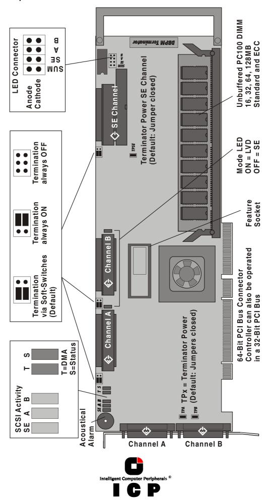
GDT7128RN, GDT7528RN and GDT7628RN Overall View
