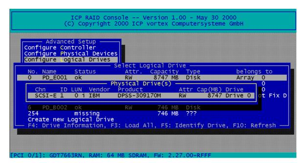
To configure and setup an new Logical Drive, select Create new Logical Drive. ICPCON displays a list of free Physical Drives (which are not already part of a Logical drive).
