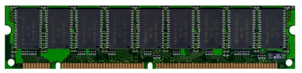
sizes. The minimum cache RAM size is 16MB. The maximum cache RAM size is 128MB. The ICP Controller provides one socket for a PC100 DIMM. The PC100 DIMM is correctly plugged into the DIMM socket of the ICP Controller if it is engaged correctly into the socket's retaining clamps and if all contacts of the PC100 DIMM are equally contacting the corresponding pins of the socket. To release an installed PC100 DIMM, carefully press the retaining clamps to the side.
