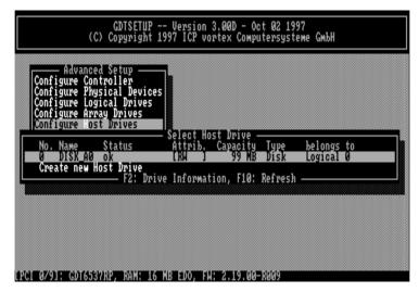
Therefore, this Host Drive has target-ID 0 and LUN 0. The formula for determining target ID and LUN from the existing Host Drive numbers yields the following possible combinations for "Direct Access Devices":
